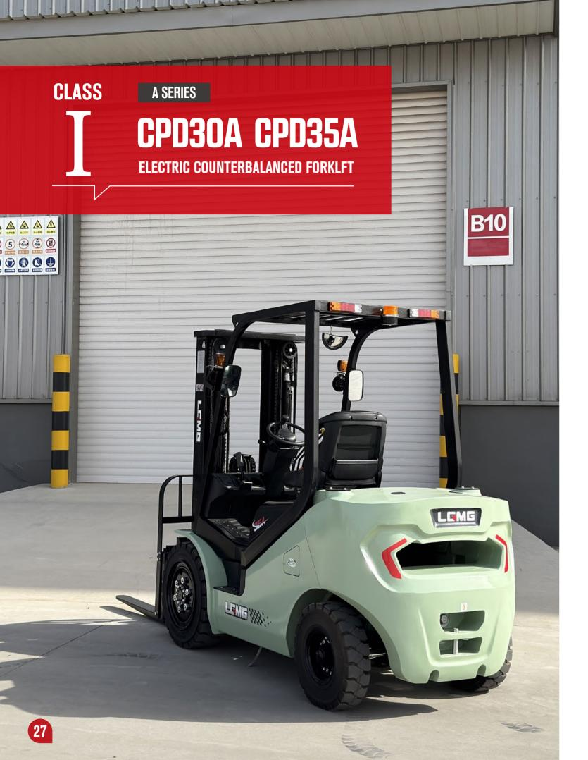
The A series new lithium battery forklift adopts internal combustion forklift's design with the strong chassis, frame, counterweight and mast. The power structure is designed to adopt LGMG electric forklift's concept, which is equipped with full AC system, Italy imported ZAPI controller, BMS control system and high quality lithium battery. This combination of IC forklift and electric forklift makes an ideal solution to reach customers' satisfaction on cost saving and environmental friendly.
